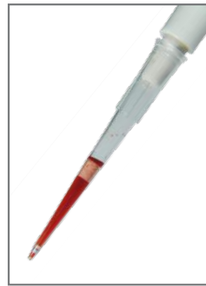
Liquid passes through conventional filter pipet tips causing cross contamination.
