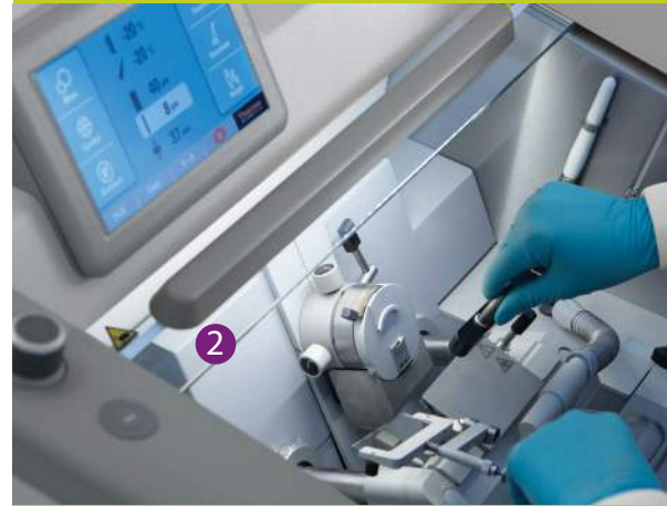
Rapid Response Temperature Control maintains sectioning surface temperature during periods of high use
