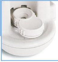
Insert Rapid fFN 10Q Cassette into the analyser.
