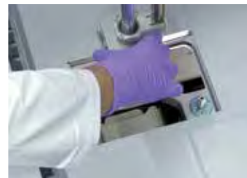
Hand guides arm to the correct centrifuge loading position below the deck using Fluent's ZeroG technology.
