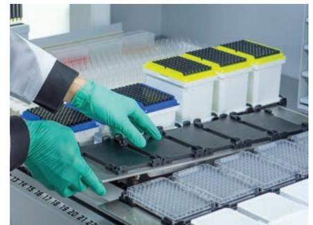
Exchange deck segments for flexible assay set-up, device integration and reconfiguration
