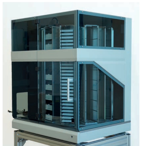
Random access to microplates or disposable tips within 15 seconds of time.
