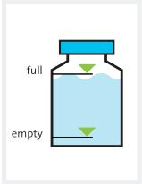
Liquid level detection (LLD) system to monitor bottle fill levels
