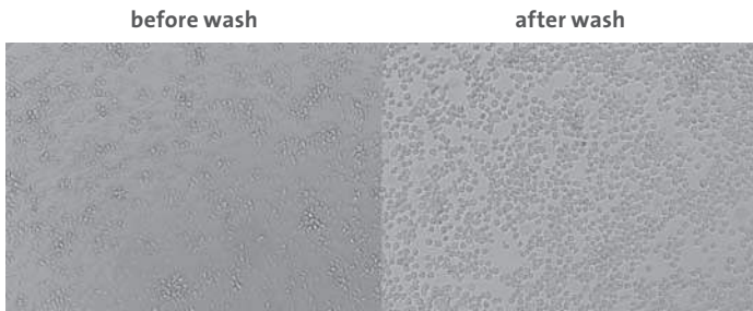
Figure 2: Washing with the HydroSpeed, indicating a gentle wash performance with almost no cell detachment.
