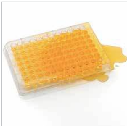
Spilling of plate caused by clogged needles
