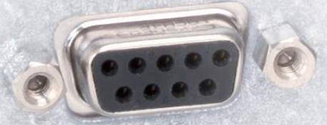
RS232 standard on all General Protocol, Advanced Protocol and Advanced Protocol Security models/sizes
