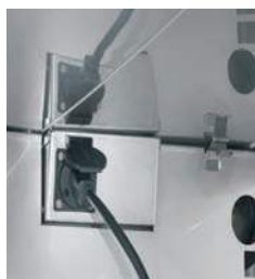
Heratherm Advanced Protocol incubators with internal socket for connection of electrical device (e.g. stirrer / shaker)
