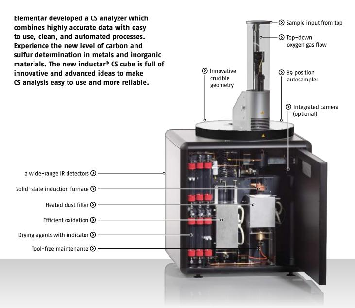
Innovative ideas combined with state-of-the-art technologies let the inductar CS cube clearly stand out from the crowd. The new construction design captures dust and debris within the ceramic crucibles. Moreover, the energy-efficient solid-state induction furnace enables high temperatures up to 2,000 °C. Combined with high-performance detectors, the inductar CS cube shows excellent accuracy and lowest possible limit of detection.
