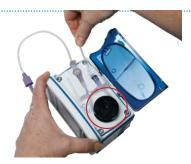
Grasp tubing at end of black retainer (where fingers are on tubing) and gently wrap tubing anti-clockwise around rotor. Pull up retainer and insert into slot. Close blue door at top of pump.
