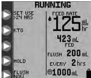
Figure 33. Running screen with the > 24 HRS of Pump Set Usage Indicator in upper left of the screen.
