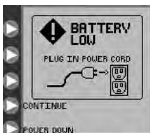
Figure 31. Battery Low error screen. Indicates that the battery must be recharged immediately.
