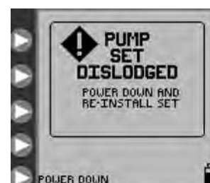
Figure 30. Pump Set Dislodged Error screen.
