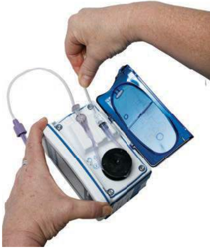
1 Load set into pump as per 'Pump Set Loading Procedure' on page 13.
