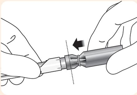
3. Place the expander cone on the tip of loading cone and push the two together – this will expand the silicone rubber band and slide it on to the base of the loading cone.
