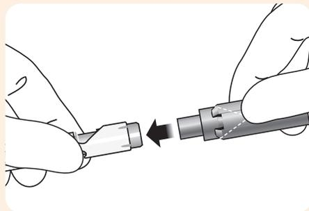
1. Insert the loading cone into the suction end of the KilRoid™ instrument.
