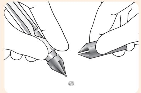
2. Place a silicone rubber band on the tip of the loading cone.
