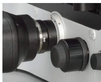
Imaging port with large 25 field number
