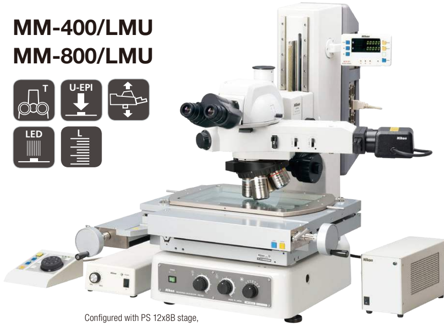
Configured with PS 12x8B stage, LV-U EPI2 universal epi-illuminator
