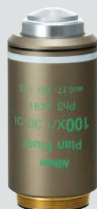
CFI Plan Fluor ADH 100x oil, NA 1.30
