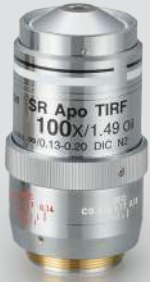
CFI SR Apo TIRF 100x oil NA 1.49, WD 0.12
