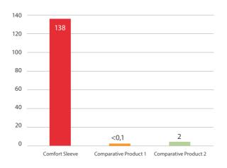
The Air permeability test measures how much breathable is a fabric quantifying the level of ease with which air passes through it. A high permeability rate indicates that air passes easily through the sleeve fabric leaving the patient leg cool and dry. The comfort sleeve material has been shown to be more permeable for air transmission than the alternative products.
