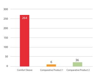
The Vapor transmission test measures the time rate for water vapor to pass through flat material surface. A high transmission rate indicates that liquid such as sweat can evaporate away from the patient leg quickly. The comfort sleeve showed the best vapor transmission rate compared to the alternative products thus resulting a highly breathable fabric.
