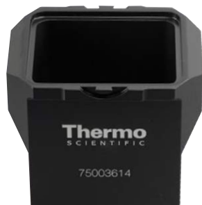
TX-750 Swinging Bucket Rotor, 90°, R max 195 mm
