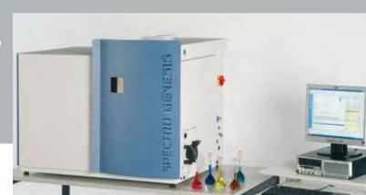
The SPECTRO GENESIS is equipped with powerful automation functions for the safe unattended analysis of a large number of samples. With an optional autosampler, several hundred samples can be processed without operator intervention. If the relevant methods are available, simply import or define a sample list.
