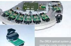
The ORCA optical system guarantees extreme stability. The CCD detectors do not need the costly cooling required for other detectors. Thermal stabilization ensures that condensing humidity cannot interfere with system performance.
