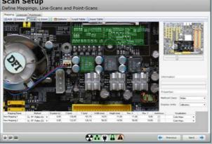
When defining line scans or mappings, the software guides you through the procedure step-by-step.
