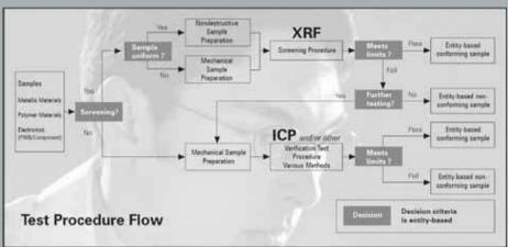
While XRF is recommended for screening measurements, the standard also recognizes that only methods that eliminate sample effects can be used as verification tests for the final confirmation of compliance. These are invariably solution techniques like ICP-OES spectrometry, and instruments like the SPECTRO ARCOS represent the state-of-the art in such
