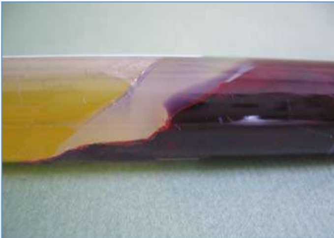
Fig. 37: Separator gel tubes centrifuged in fixed-angle centrifuges and transported horizontally. Jolts could break the gel barrier.
