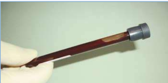
Fig. 27: Air bubble as indicator for mixing
