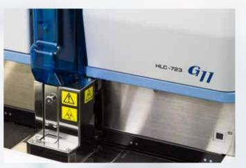
"What I find user friendly is the rack rotation switch. In this way the analyser knows when the last sample has been analysed and will go directly in wash mode. Afterwards there is a customisable timer to power off the analyser."
