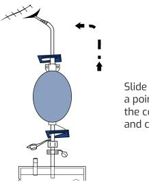
Slide clam p to a point just b elow the connec tion and close off.
