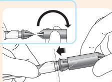
4. Withdraw the expander cone from the loading cone, rotate the expander cone through 180°, presenting the open end of the expander cone to the loading cone. Push the silicone rubber band on to the suction end of the instrument.
