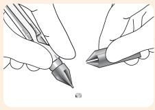
2. Place a silicone rubber band on the tip of the loading cone.
