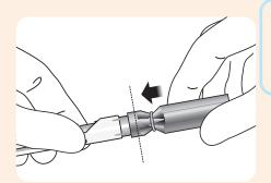
3. Place the expander cone on the tip of loading cone and push the two together – this will expand the silicone rubber band and slide it on to the base of the loading cone.
