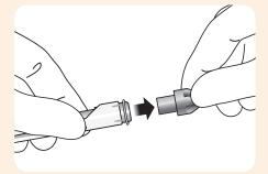
5. Remove the loading cone – the silicone rubber band is now mounted on the suction end and the instrument is ready to use.
