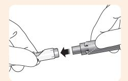
Insert the loading cone into the suction end of the KilRoid™ instrument.
